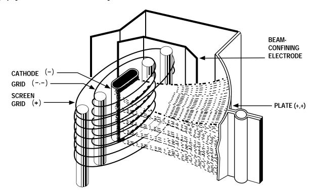
Structure of a 6L6 / 5881 Beam Power Pentode.
